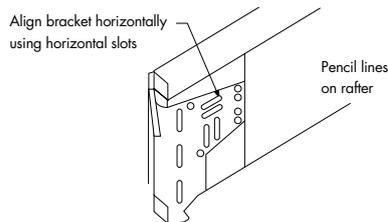
4. Fix 2 rafter brackets to the end rafters on the marked lines.
